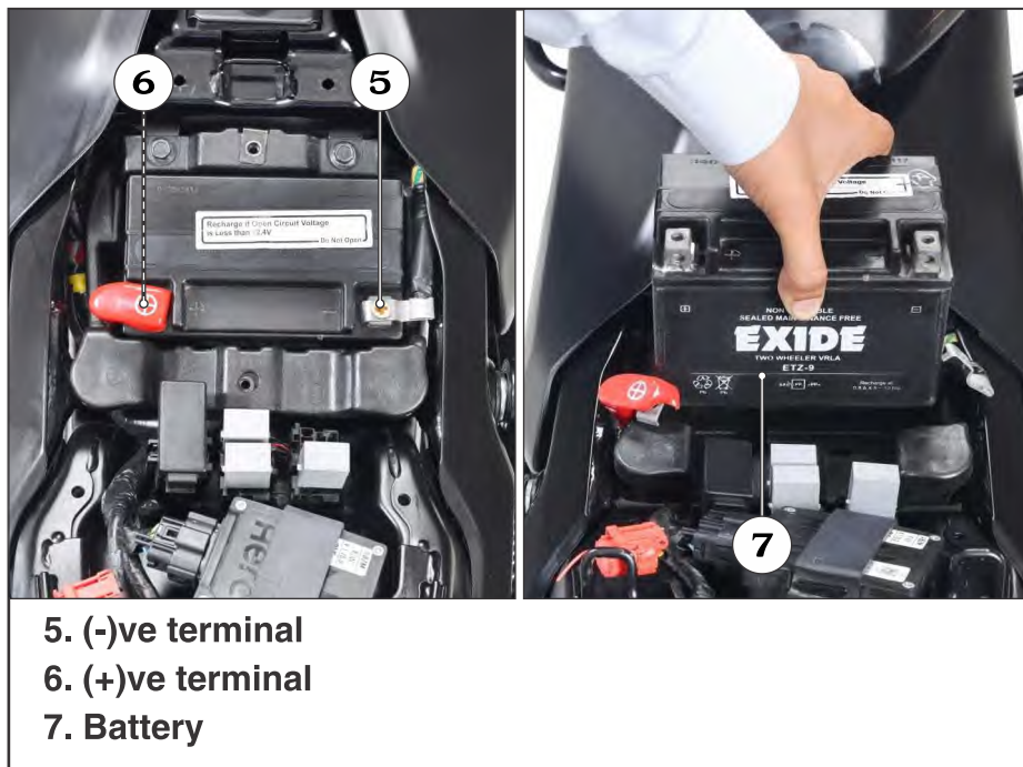
Figure 83. Battery removal
