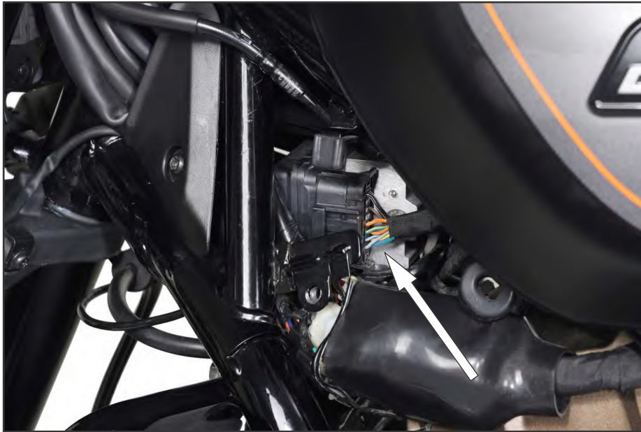
Figure 11. ABS Module (HECU) (located below Fuel tank)
