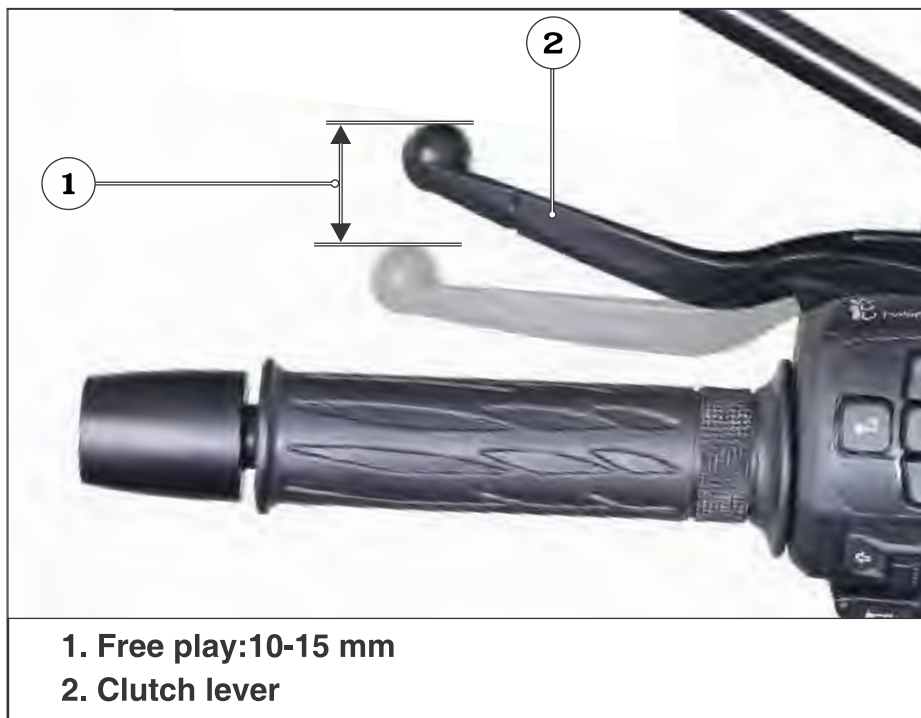
Figure 66. Clutch lever free play
